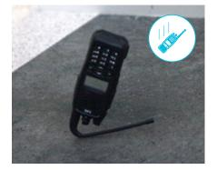
We drop them from 6 feet onto concrete – that's 50% higher than the MIL-STD-810G specification test. We drop each radio dozens of times from different angles, ensuring the durability of everything from battery and antenna fittings to internal components and the screen. MIL-STD-810G refers to protection against: Low pressure, Low temperature, High temperature, Temperature shock, Solar radiation, Rain, Humidity, Salt fog, Dust, Vibration, and Shock.
